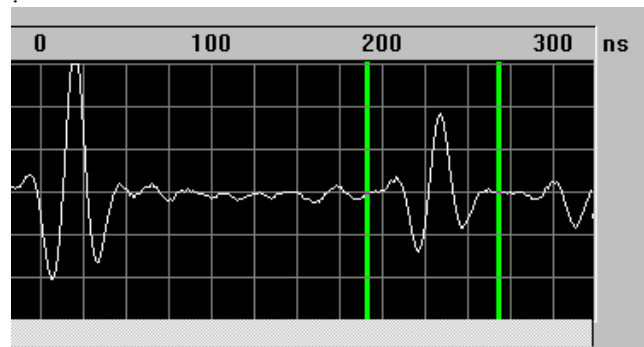
Figure 7: A-scan displaying typical waveforms (pulses) in the time domain.
