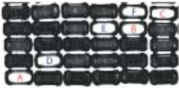
Figure 3: Acoustic Image of Same Capacitors in Figure 2, after “Dark” Capacitors Rotated 90°—Three More Capacitors Seen with Internal Defects (D, E, and F)
