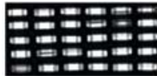
Figure 4: LOBE (Loss Of Back Echo) Image Made at Same Time as Figure 2—All Six Defective Capacitors Can Be Identified
